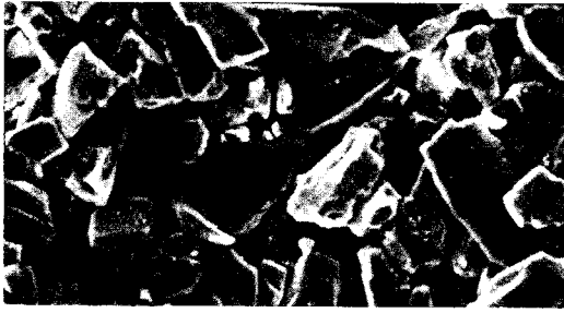
Fig. 11: Aluminium oxide grit 280/36 200x magnification, particle count 100%, hardly any overlapping particles.
