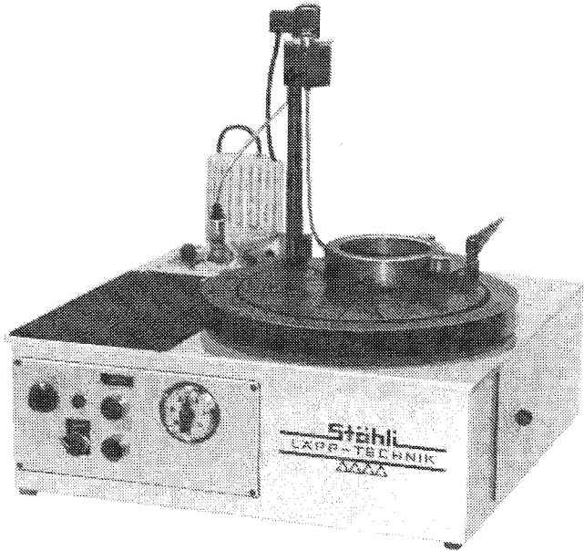
Figure 14: Bench-type lapping machine for hand lapping and machine lapping, equipped with lapping medium pump, variable distribution head, variable-speed drive and timer.
