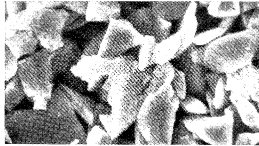
Fig. 12: Silicon-carbide grit 800/ 6.5. 2000x magnification, particle count 150%, at least 50% overlapping grains.
