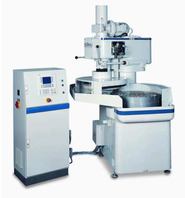
Figure 12: ZL 501, Hahn & Kolb System series with loading/unloading table and pivot arm
