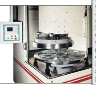
Flathoning machines are unlike conventional fixed abrasive grinders used for sizing components. Clean lapping far exceeds the 0.0002-in to 0.0003-in tolerances of conventional grinders. A smaller machine can finish up to 100-150 inserts within 7-8 minutes, a rate of 700-1000 parts per hour.
