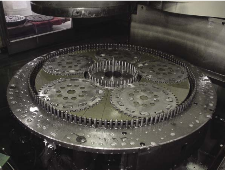
Multiple workpieces are processed at a time using discs to hold and orient the parts.
